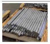
To maintain consistency in material, all Rolled Alloys stocked 416R round bar meets the following criteria:
